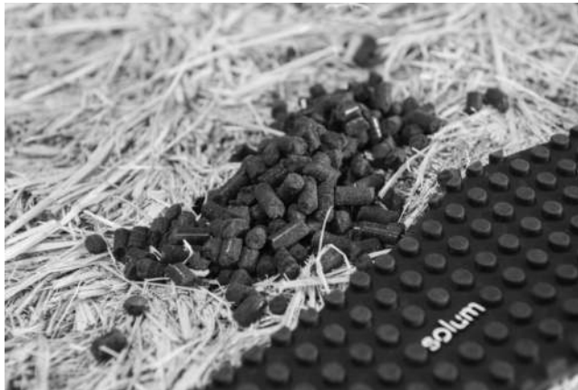
That raw fiber gets ground into a fine powder, turned into pellets and later pressed into the sole.
