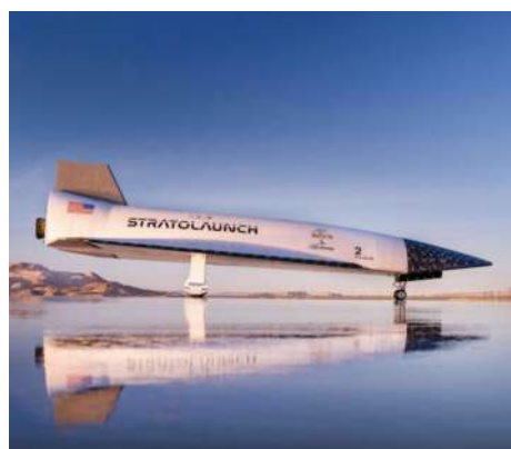
Talon-A2 is a recoverable autonomous hypersonic testbed designed for repeated air launch.
