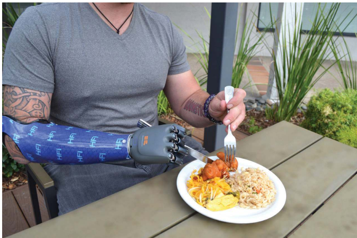
Army Capt. Carey Duval tries out his BrainRobotics hand during a meal. BrainRobotics has created an AI prosthetic that reads minute muscle signals and responds to create a variety of hand gestures.
