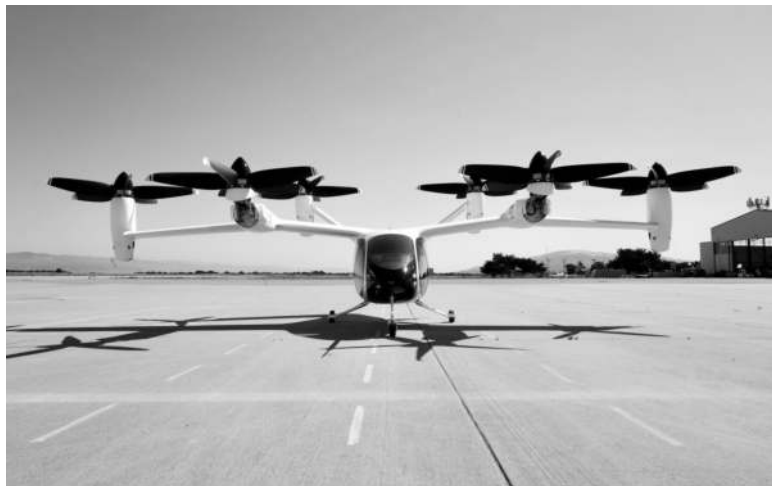
An “electric vertical take-off and landing” aircraft built by Joby Aviation is parked at an airfield in Marina.
