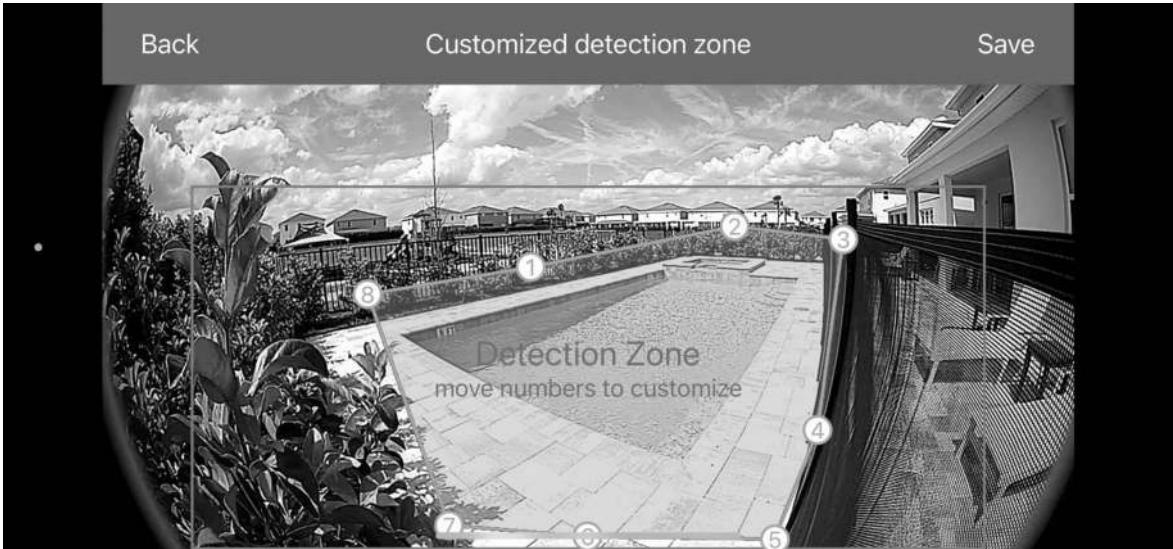
The SwamCam artificial intelligence-powered drowning detection system has a fish-eye lens with a 160-degree field of view, records in 1080p, has night vision and works in temperatures ranging from minus 4 degrees up to 140 degrees Fahrenheit.
