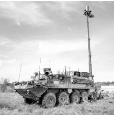
A U.S. Army Stryker mounted with a Tactical Electronic Warfare System-Infantry provides support to soldiers.
