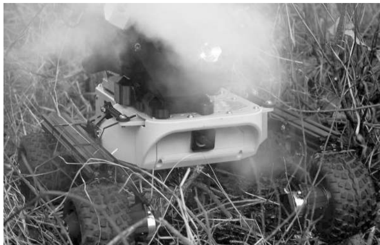
With its decoy weapon, Gereon can simulate machine-gun fire using a loudspeaker and LED muzzle flash. Additional components could add lasers and other sensor equipment to the vehicle base.
