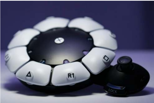
The Sony Access controller can rest on a table or wheelchair tray or be mounted on a tripod. Its buttons and thumbsticks are also customizable.
