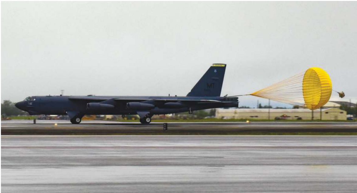
A drogue parachute helps a B-52H Stratofortress slow down upon landing at Joint Base Elmendorf-Richardson, Alaska, on July 17.
