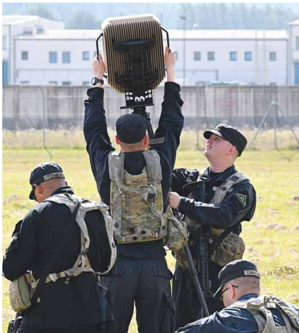
Soldiers with 1st Battalion, 4th Infantry Regiment set up an EchoShield radar system used to detect and track drones at Hohenfels. The radar is one of several new electronic warfare tools the opposition force is fielding this year, along with jamming systems designed to disrupt enemy communications and disable drones.
