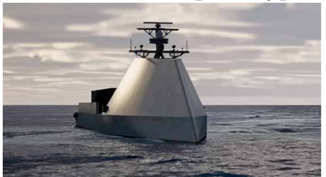
Huntington Ingalls Industries An artist rendering of Romulus, a Medium Unmanned Surface Vessel, designed by Huntington Ingalls Industries. HII is among seven companies chosen by the Navy to submit MUSV prototypes.
