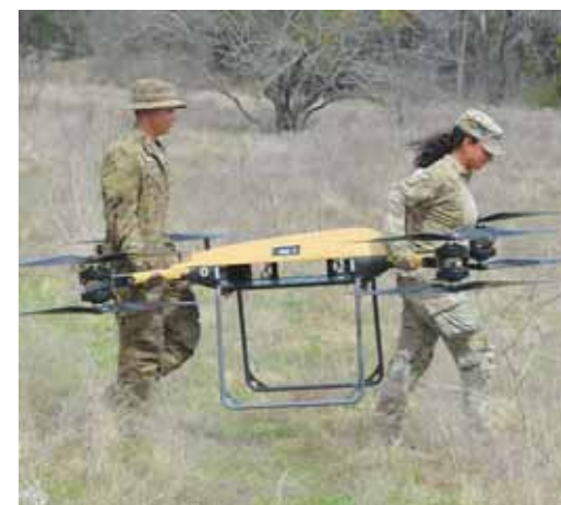
Soldiers from the 36th Engineer Brigade carry a TRV-150 unmanned aircraft capable of moving up to 150 pounds during training at Fort Hood.
