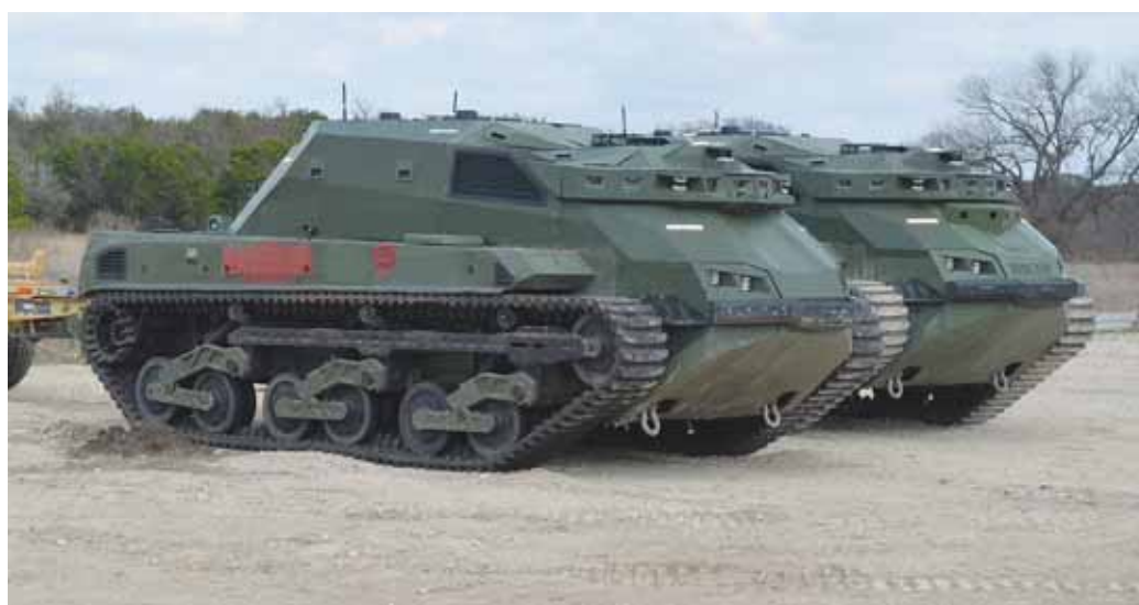
The 36th Engineer Brigade received two M5 RACER unmanned vehicles to breach obstacles without soldiers directly on the line from a retired Defense Advanced Research Projects Agency program.
