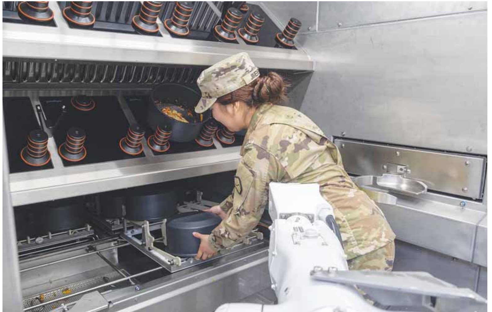
PHOTOS BY ALEJANDRO CARRASQUEL/Stars and Stripes Army Pfc. Ximena Jimenez, a culinary specialist with 19th Expeditionary Sustainment Command, uses the autonomous field kitchen at Camp Carroll, South Korea. The containerized kitchen can produce between 100 and 120 meals per hour, the command’s food adviser said.
