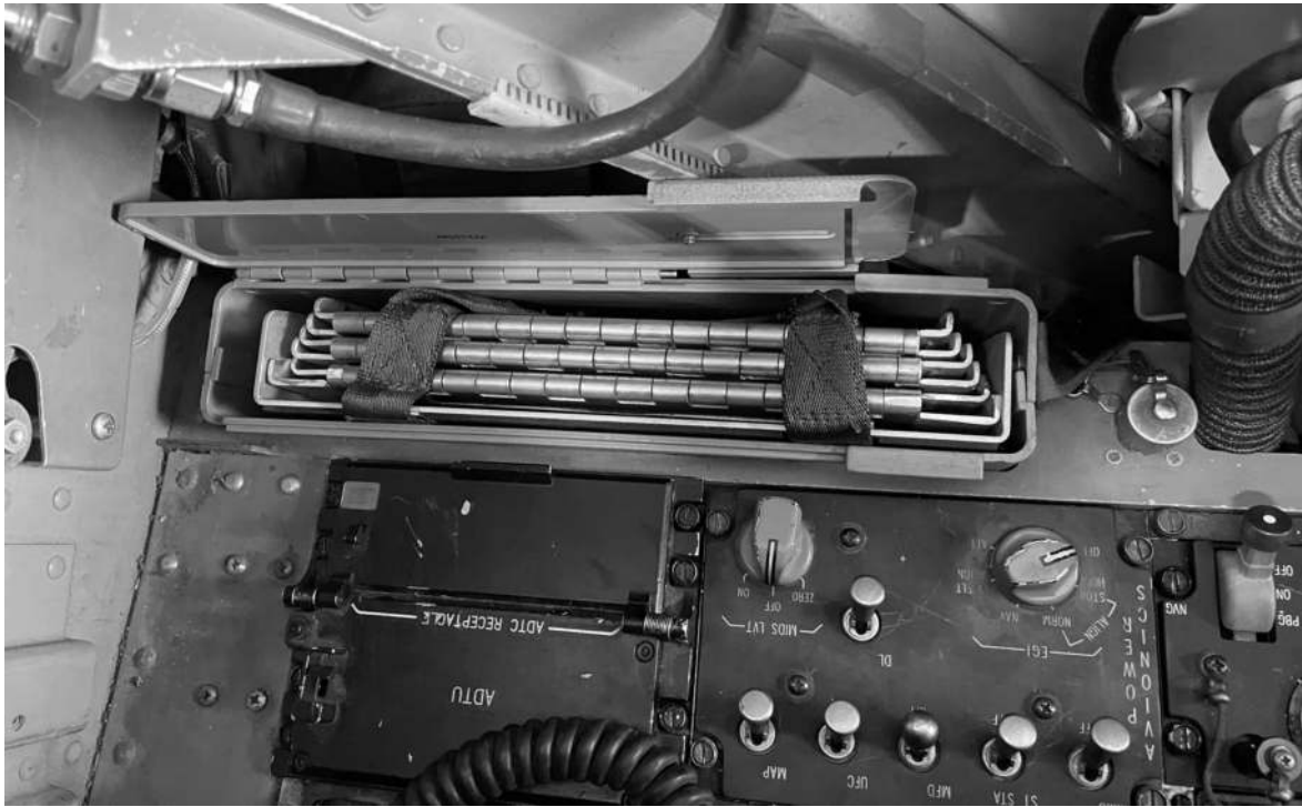
A prototype collapsible ladder for the F-16 Viper is stored in the cockpit map case. The idea for the ladder came from Maj. Nicholas Atkins, an F-16 pilot at Aviano Air Base in Italy.
