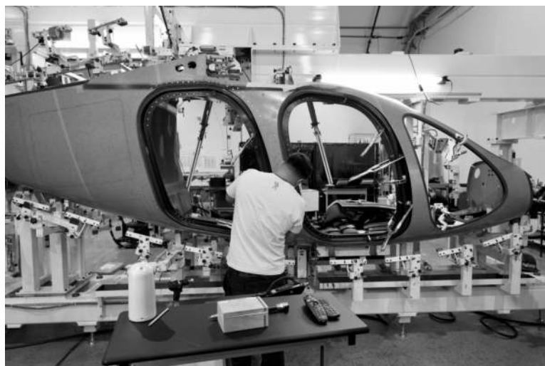
A Joby Aviation employee works on the assembly of an eVTOL aircraft in Marina.
