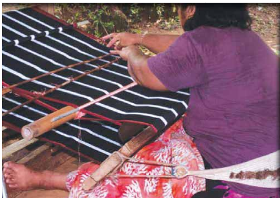
Traditional backstrap loom made and used by "Remathau" family, or Outer Islanders, of Yap. The strap is made of coconut fiber and lasts for many years. The loom is made of local mahogany wood and bamboo. Photo by Joyce McClure
