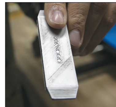
Reynolds holds a .50 caliber machine gun gauge made by their new metal 3D printer.
