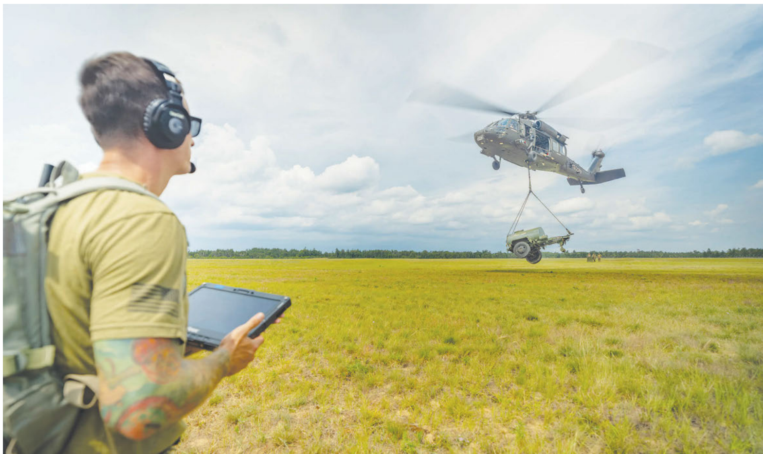
A National Guard soldier uses a tablet to command the Sikorsky OPV Black Hawk to autonomously transport a 2,900-pound water buffalo sling load for the first time during the Northern Strike exercise in Michigan in August.
