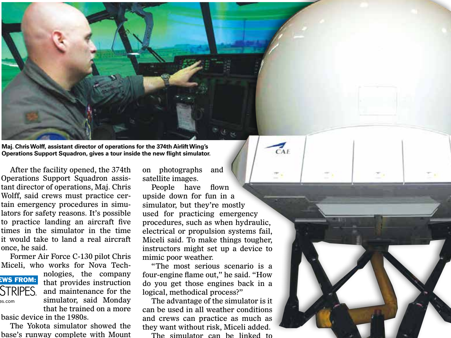
A curved mirror reflects five video feeds through the front windows while a hi-fi sound system mimics engine noise and electronic legs tilt the cabin to give those inside the sensation of motion. Photos by Theron Godbold, Stars and Stripes
