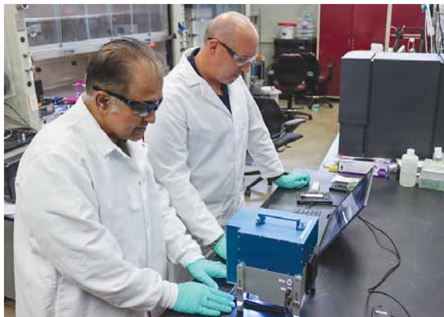
Research scientists Dr. Jason Guicheteau and Dr. Ashish Tripathi use the Portable Microscopy Chemical Detection System to test samples containing trace amounts of particles and identify the substance.
