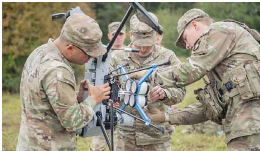
Soldiers attach a 3D-printed grenade dropper on a C100 drone for target practice at Hohenfels, Germany.
