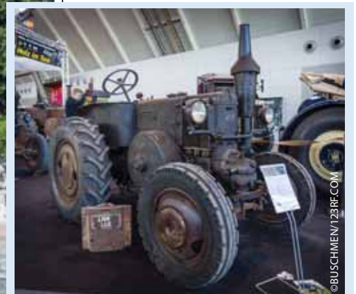
The tractor Lanz Bulldog D7511 (two-stroke, hot bulb engine), manufactured by Heinrich Lanz AG in Mannheim, 1935.
